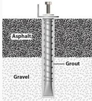
weight to 12 oz of EPX2 powder by weight. See [Anchor installation manual](#) for details and the correct mixing procedure.
