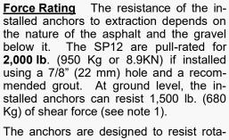
tional torque. Torque is generated when tightening the bolt into the anchor. Excessive torque will break the bond between the anchor and the asphalt, or may damage the internal thread or weld in the anchor. The SP12 is rated for a torque of 200 lb-in.
